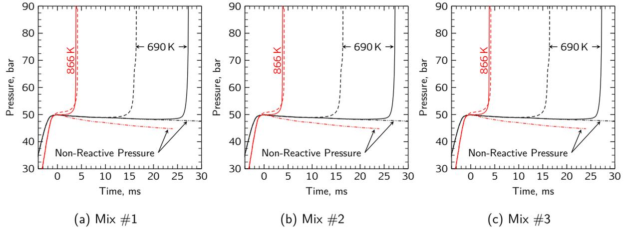
**Figure 5.8:** Comparison of selected simulated and experimental pressure traces at  $P_C = 50$  bar. Red lines indicate that the pressure profile of the reactive simulation deviates from the non-reactive case prior to EOC. Solid lines: experiment; dashed lines: reactive simulation; dot-dot-dashed lines: non-reactive simulation.
