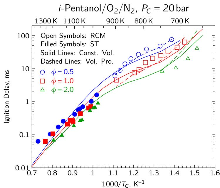
**Figure 4.3:** ST and RCM ignition delay times published in Tsujimura et al. [77] at 20 atm compared with model predictions by the model from Sarathy et al. [75]. The RCM studies were conducted as part of this thesis.
