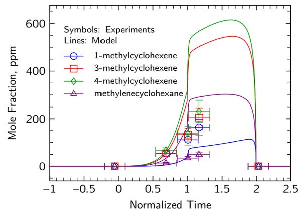
**Figure 5.13:** Comparison of the present model with the sampling experiments for the isomers of methylcyclohexane.
