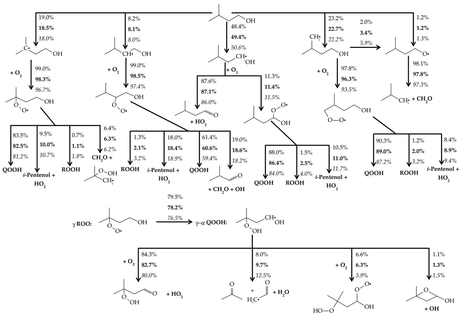
**Figure 4.10:** Reaction path analysis for *i*-pentanol at 800 K, 20 atm, and three equivalence ratios, based on constant-volume adiabatic simulations. Plain text:  $\phi = 0.5$ . Bold text:  $\phi = 1.0$ . Italic text:  $\phi = 2.0$ . The species flux is integrated up to 20% fuel consumption.
