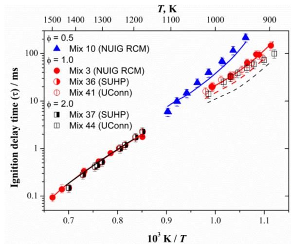
**Figure E.9:** Ignition delays of propene with 4% O<sub>2</sub> at 40 atm for three equivalence ratios
