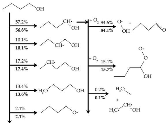
**Figure 3.19:** Pathway analysis for simulations of *n*-butanol at temperature of 750 K, in stoichiometric air, using the mechanism of Sarathy et al. [154]. Percentages in normal text represent an initial condition of 15 bar; bold text is for 30 bar.
