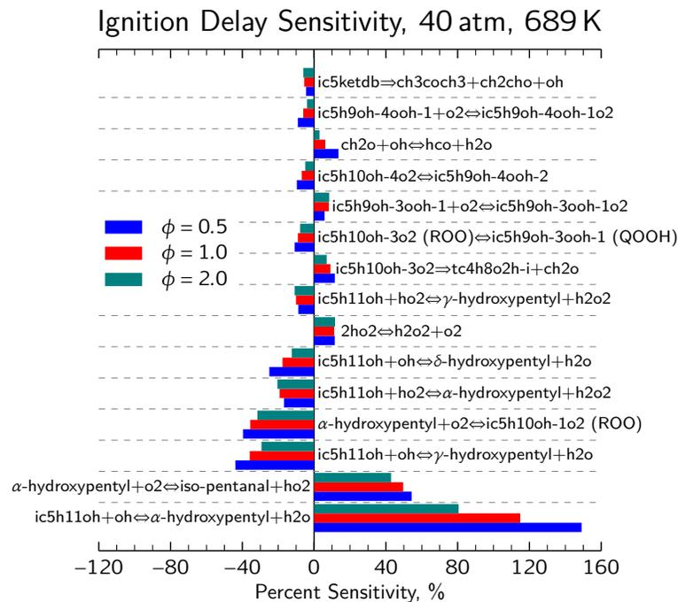
**Figure 4.9:** Sensitivity of the ignition delay to changes in the reaction rate coefficients for three equivalence ratios. Initial conditions for constant-volume adiabatic simulations are 689 K and 40 atm.
