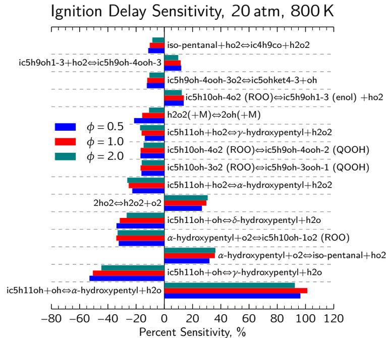
**Figure 4.8:** Sensitivity of the ignition delay to changes in the reaction rate coefficients for three equivalence ratios. Initial conditions for constant-volume adiabatic simulations are 800 K and 20 atm.
