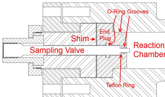
**Figure B.2:** Schematic of the GSV assembled into the reaction chamber showing the position of the sealing o-rings and the protrusion of the poppet face.
