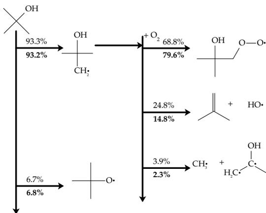
**Figure 3.21:** Pathway analysis for simulations of *t*-butanol at temperature of 750 K, in stoichiometric air, using the mechanism of Sarathy et al. [154]. Percentages in normal text represent an initial condition of 15 bar; bold text is for 30 bar.
