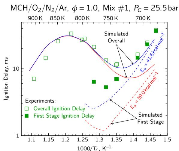
**Figure 5.10:** Comparison of mechanism performance with the activation energy of ketohydroperoxide decomposition set at  $41.6 \text{ kcal mol}^{-1}$  (blue) and  $39.0 \text{ kcal mol}^{-1}$  (red). Experimental ignition delays are shown in green symbols.
