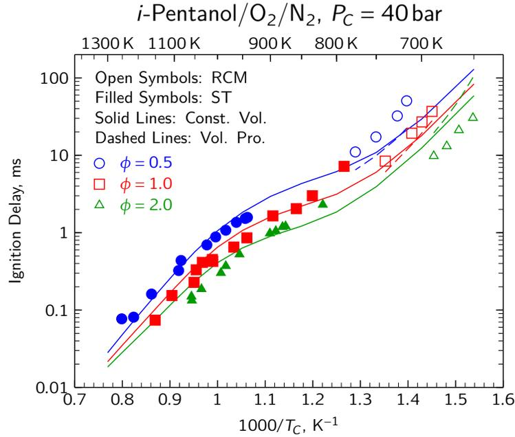
**Figure 4.4:** ST and RCM ignition delay times published in Sarathy et al. [75] at 40 atm compared with model predictions by the model from Sarathy et al. [75]. The RCM studies were conducted as part of this thesis.
