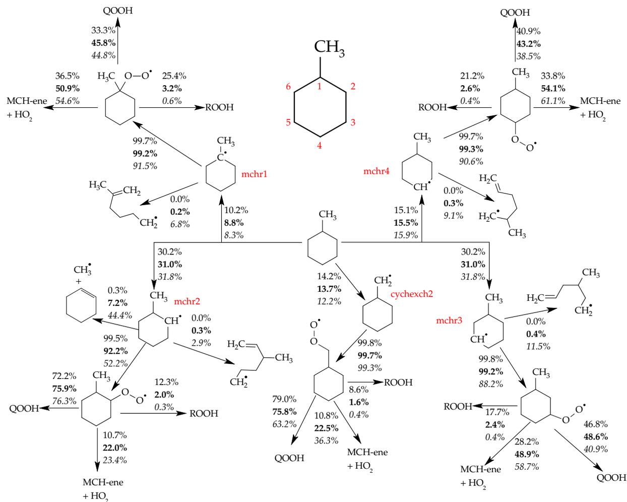
**Figure 5.14:** Path analysis of MCH combustion. Initial conditions are 25.5 bar and Mix #1 ( $\phi = 1.0$ ) and 700 K (plain text), 800 K (bold text), 900 K (italic text). Note that not all possible reaction pathways are shown for each species.
