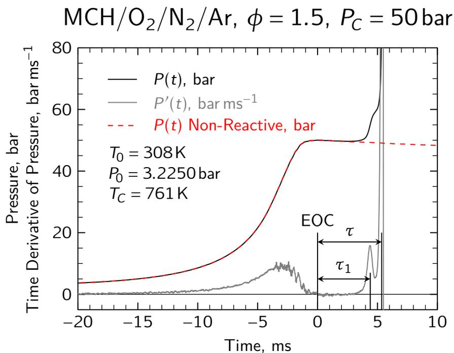
**Figure 2.3:** Representative pressure trace indicating the definition of the first stage and overall ignition delays and the corresponding non-reactive pressure trace. EOC stands for End of Compression.
