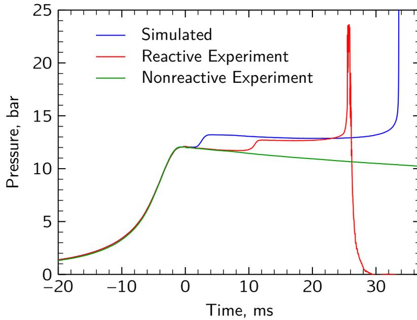
**Figure 5.11:** Pressure traces of the experiments with the RSA installed compared with the simulated pressure trace.
