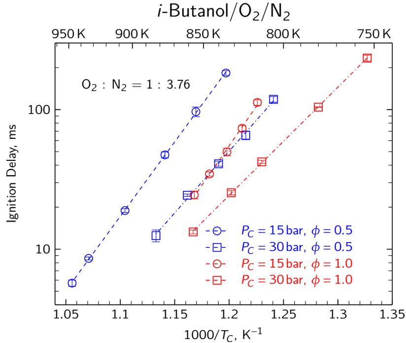
**Figure 3.9:** Comparison of the experimentally measured ignition delays of *i*-butanol at two compressed pressures,  $P_C = 15$  bar (circles) and  $P_C = 30$  bar (squares), and two equivalence ratios,  $\phi = 0.5$  (blue) and  $\phi = 1.0$  (red).
