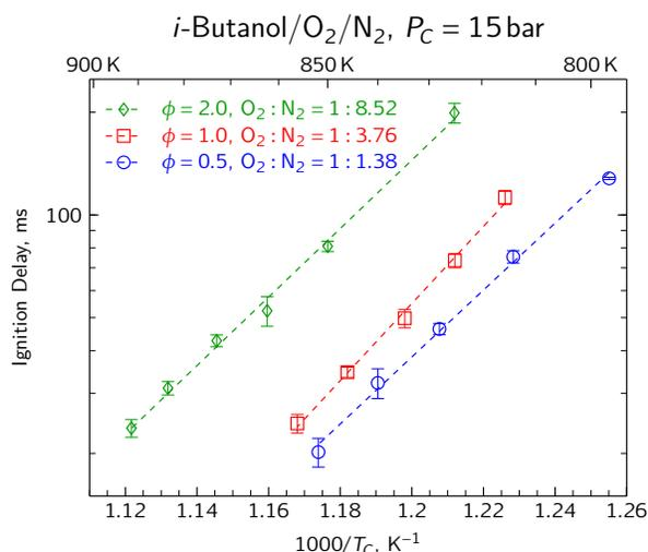
**Figure 3.10:** Comparison of the experimentally measured ignition delays of *i*-butanol at three equivalence ratios and  $P_C = 15$  bar. The equivalence ratio is changed by varying the initial oxygen mole fraction at constant initial fuel mole fraction.
