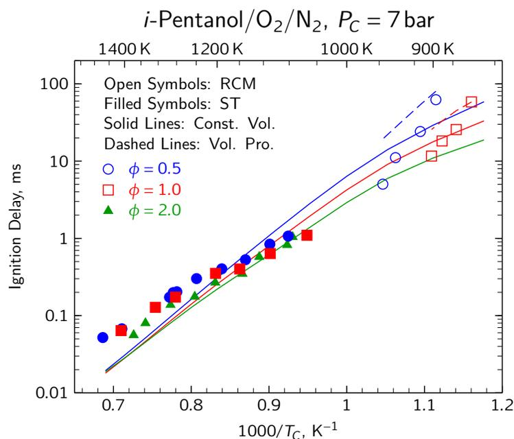
**Figure 4.2:** ST and RCM ignition delay times published in Tsujimura et al. [77] at 7 atm compared with model predictions by the model from Sarathy et al. [75]. The RCM studies were conducted as part of this thesis.
