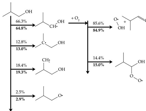
**Figure 3.22:** Pathway analysis for simulations of *i*-butanol at temperature of 750 K, in stoichiometric air, using the mechanism of Sarathy et al. [154]. Percentages in normal text represent an initial condition of 15 bar; bold text is for 30 bar.
