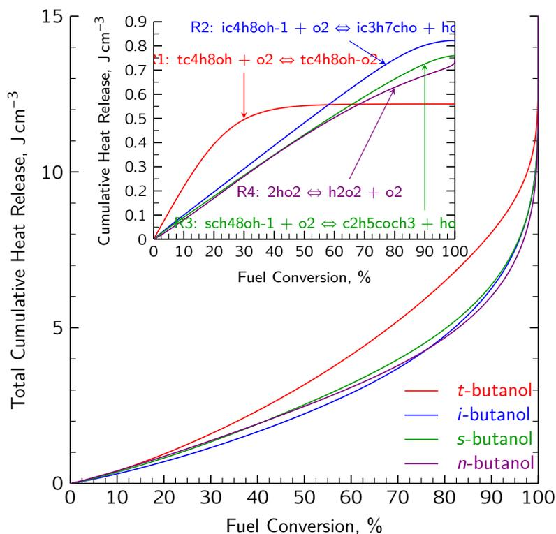
**Figure 3.23:** Total cumulative heat release and cumulative heat release by important reactions (inset) as a function of fuel consumption from a simulation using the mechanism of Sarathy et al. [154] with initial conditions of 750 K and 30 bar, in stoichiometric air. See Fig. 3.24 for definitions of reactions in the inset.
