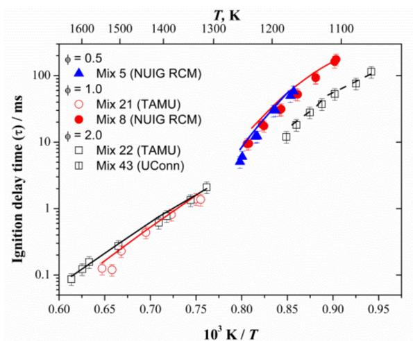
**Figure E.8:** Ignition delays of propene with 4% O<sub>2</sub> at 10 atm for three equivalence ratios
