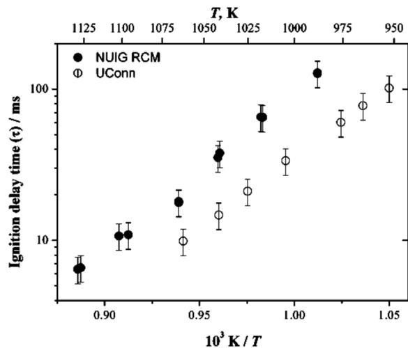
**Figure E.2:** Comparison of ignition delays of propene measured in the UConn and NUI Galway RCMs.  $P_C = 10\text{ atm}$ ,  $\phi = 1.0$ ,  $12\% \text{ O}_2$ .
