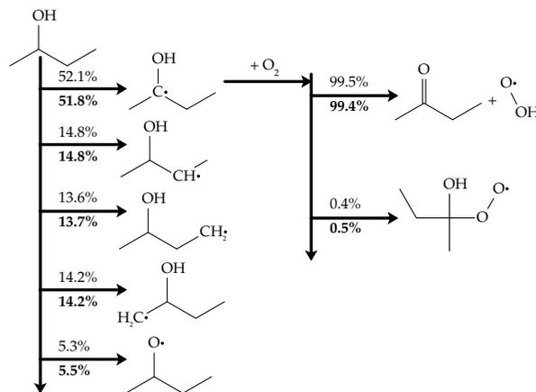
**Figure 3.20:** Pathway analysis for simulations of *s*-butanol at temperature of 750 K, in stoichiometric air, using the mechanism of Sarathy et al. [154]. Percentages in normal text represent an initial condition of 15 bar; bold text is for 30 bar.
