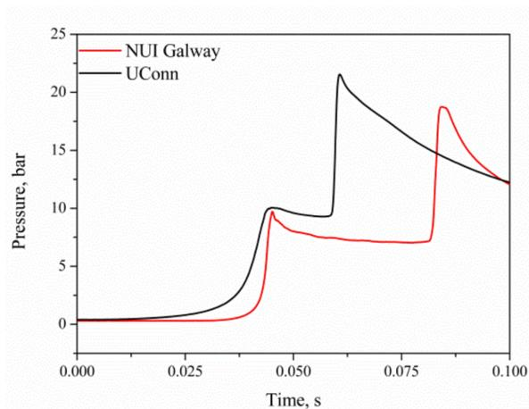
**Figure E.1:** Comparison of pressure traces between the UConn and NUI Galway RCMs.  $P_C = 10\text{ atm}$ ,  $T_C \approx 1040\text{ K}$ ,  $\phi = 1.0$ ,  $12\% \text{ O}_2$ .
