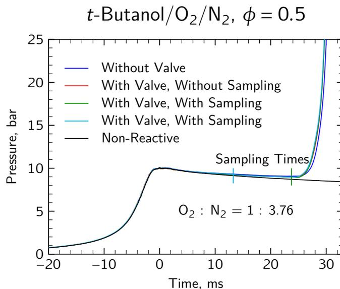
**Figure B.3:** Representative pressure traces from RCM experiments with and without the GSV present, and with and without sampling occurring. Two sampling times are shown. The corresponding non-reactive pressure trace is also shown.
