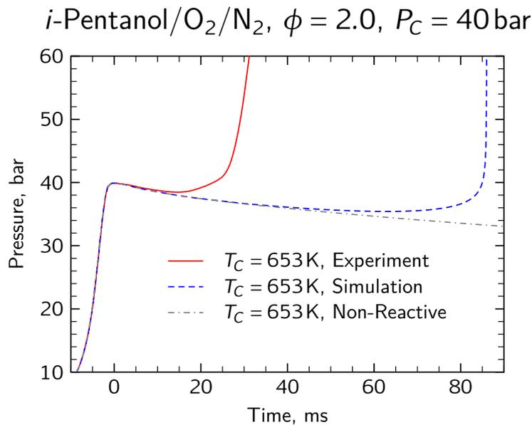
**Figure 4.7:** Experimental reactive (red, solid), simulated reactive (blue, dashed), and experimental non-reactive (gray, dot-dashed) pressure profiles at 40 atm for rich *i*-pentanol/air mixtures.
