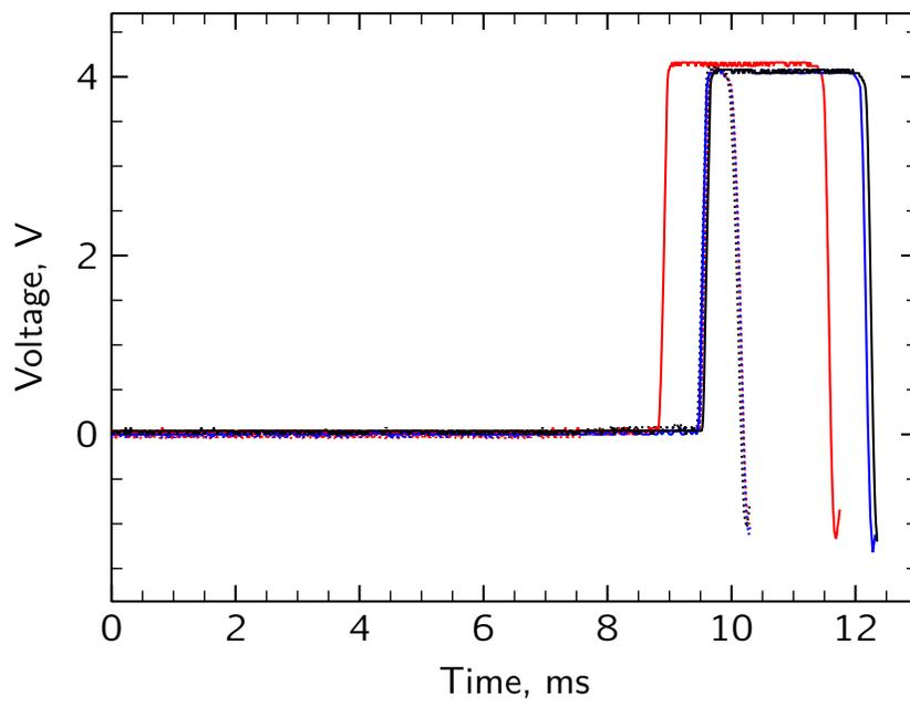
**Figure B.5:** Representative voltage traces from three runs each of two COG times: dotted: 0.8 ms; solid: 2.5 ms.
