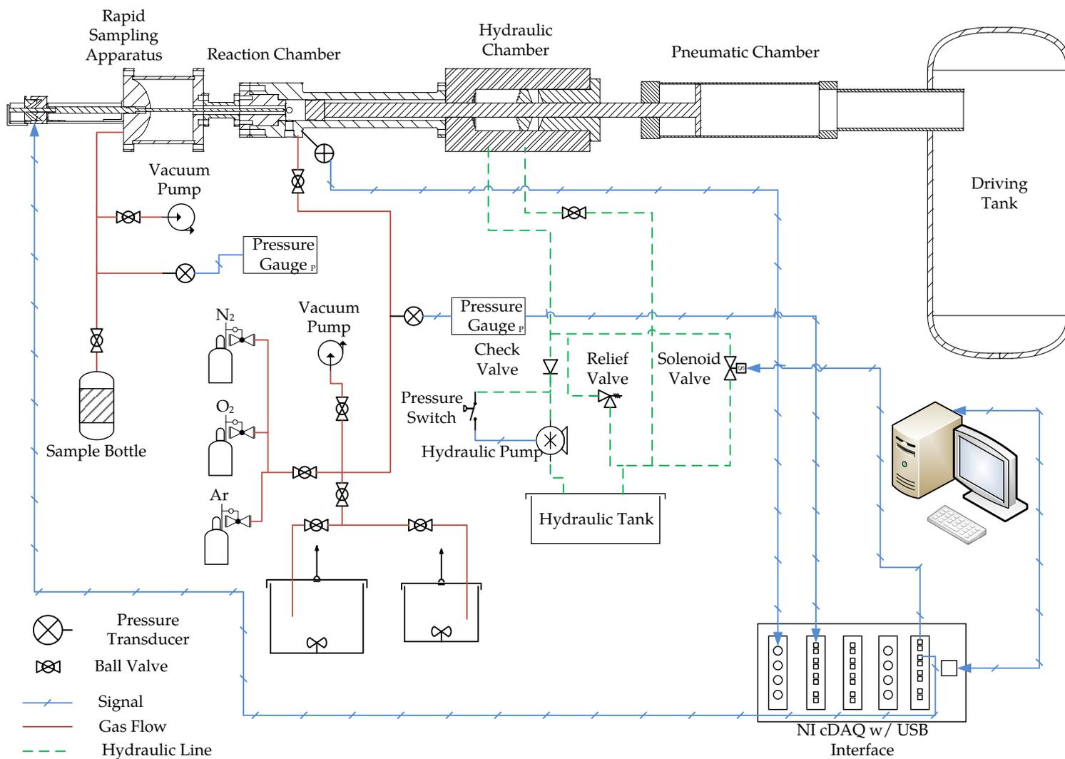
Figure 2.2: Schematic of the RCM. Not to scale
