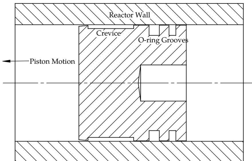
**Figure 2.4:** Creviced piston installed in the present RCM.
