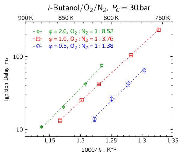
**Figure 3.11:** Comparison of the experimentally measured ignition delays of *i*-butanol at three equivalence ratios and  $P_C = 30$  bar. The equivalence ratio is changed by varying the initial oxygen mole fraction at constant initial fuel mole fraction.
