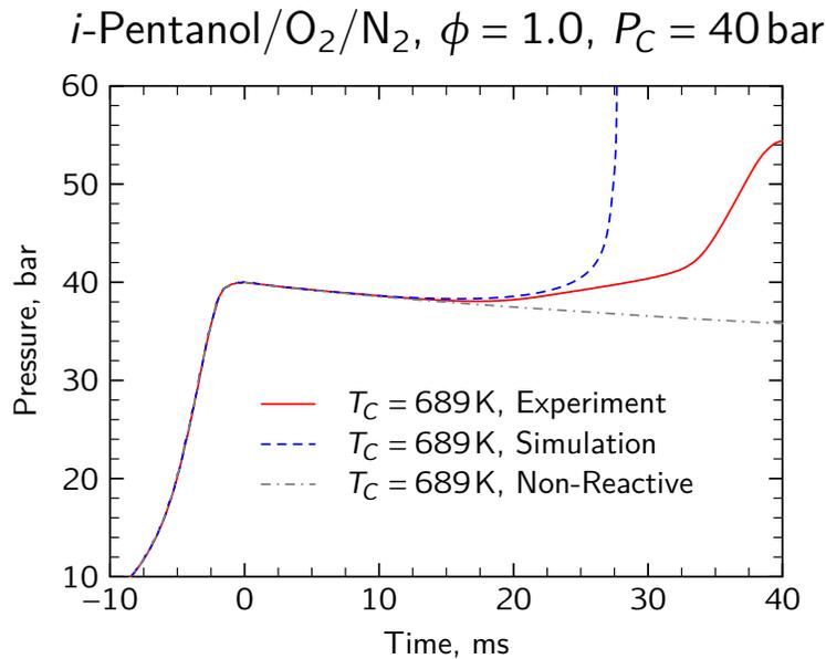
**Figure 4.6:** Experimental reactive (red, solid), simulated reactive (blue, dashed), and experimental non-reactive (gray, dot-dashed) pressure profiles at 40 atm for stoichiometric *i*-pentanol/air mixtures.
