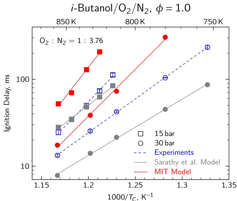
**Figure 3.16:** Comparison of VPRO simulations using the kinetic mechanism of Sarathy et al. [154] (gray) and the MIT mechanism [66] (red) with the experimental ignition delay results (blue) for stoichiometric mixtures of *i*-butanol in air at  $P_C = 15$  bar (squares) and  $P_C = 30$  bar (circles).
