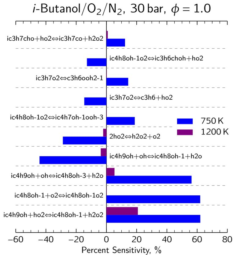
**Figure 3.26:** Linear brute force sensitivity analysis of the ignition delay with respect to the A-factors of the listed reactions in the mechanism from Sarathy et al. [154]. Positive quantities indicate the ignition delay is increased when the A-factor is halved.
